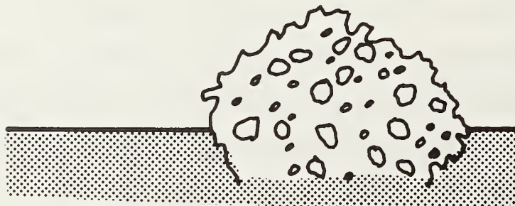
Figure 3.5. Some Theoretical Models of Polish-Resistant Aggregates [James 1968]
